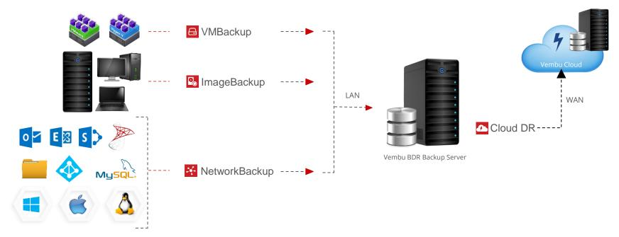
Setup DR site in your local environment and backup via LAN connections and send another copy of backup data to Vembu Cloud via WAN connection by signing up to Vembu CloudDR service
