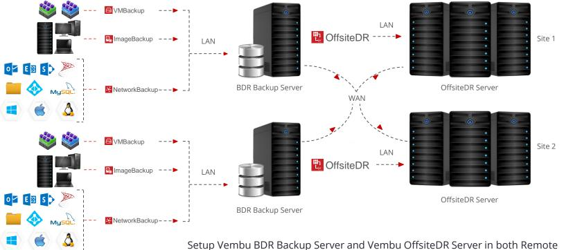
Setup Vembu BDR Backup Server and Vembu OffsiteDR Server in both Remote office and Branch office and sync backup data between both the locations
